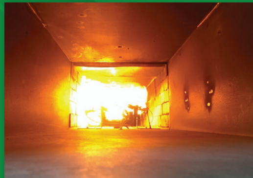
STEINER TUNNEL TESTING FOR FLAME & SMOKE DEVELOPMENT
