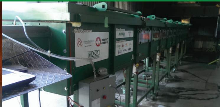
STEINER TUNNEL TESTING FOR FLAME & SMOKE DEVELOPMENT
