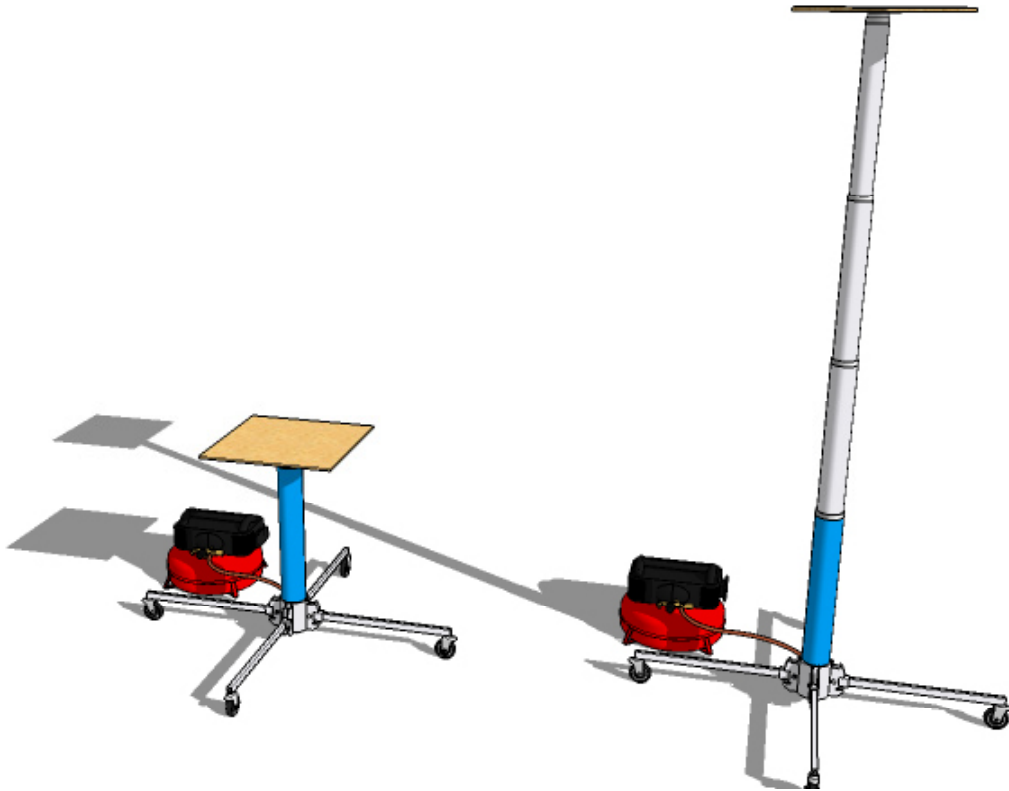
Dia. 4 Genie ceiling lift.
