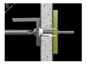
Place item over flange. Insert bolt through item and tighten until flush against item.
