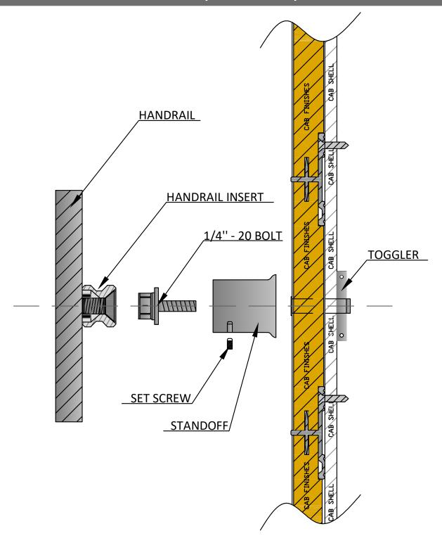
**Dia. 1** Attaching standoffs to handrail.
