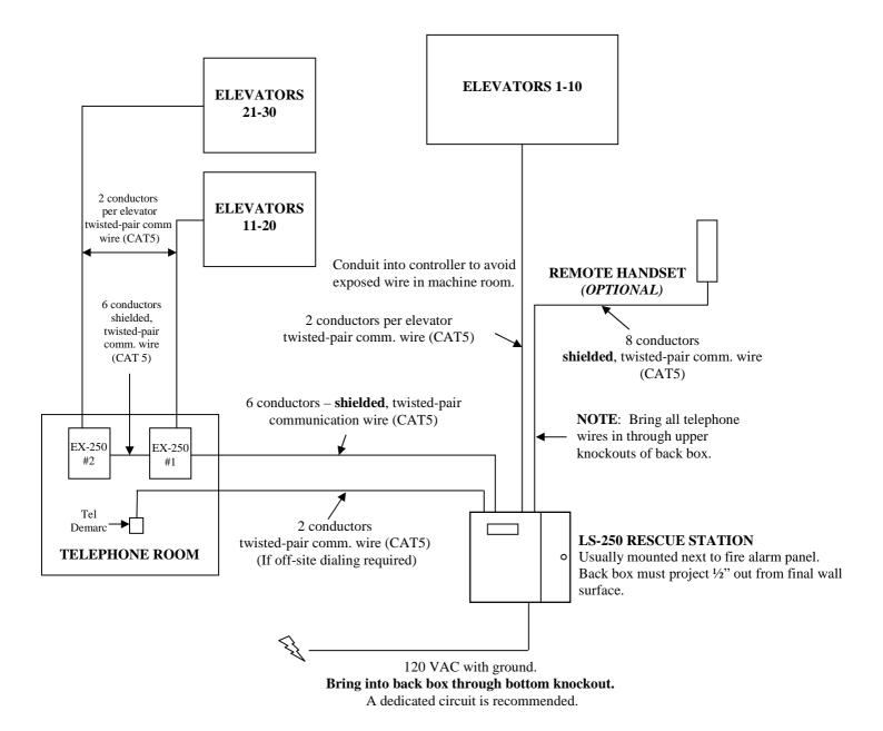
NOTE: This wiring diagram supercedes the wiring diagram provided with the LS-250 Rescue Station.
